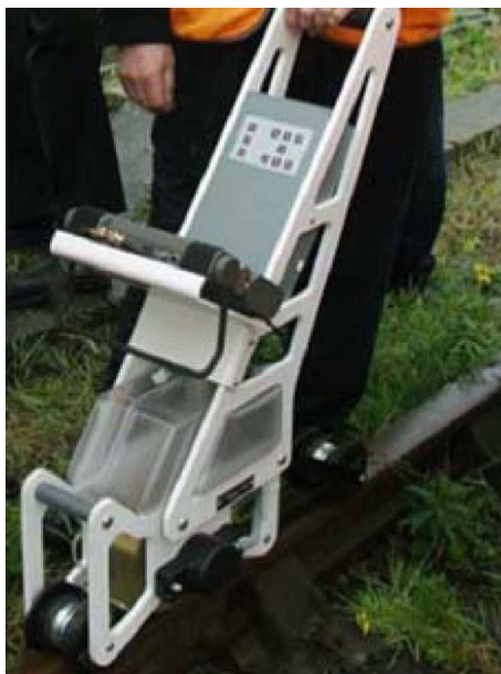
Fig. 7 Example of an ultrasonic walking stick (taken from reference [17])
