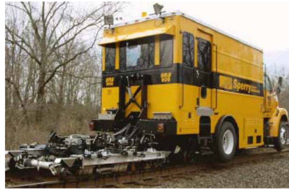
Fig. 8 Hi-rail ultrasonic-MFL inspection vehicle (taken from reference [17])
